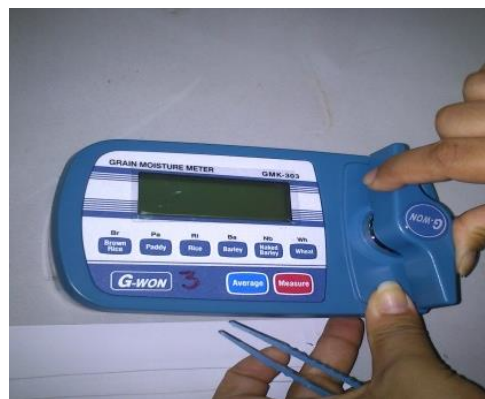
Gambar 4. Moisture meter tipe Resistansi (G-won meter)
